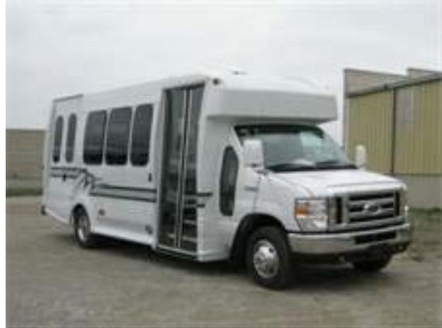
The proposed procurement will be for 23 Turtle Top “Odyssey” models (pictured), to be built on Ford chassis with three varying seating capacities on each vehicle (using foldaway seating) of:
