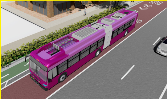
Frequent headways and specially branded, hybrid/electric, low-floor buses for level boarding with amenities such as on-board wi-fi, bike storage, etc.
